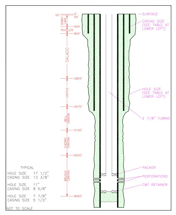
FIGURE 2 Typical Well Structure and General Stratigraphy Near the WIPP Site
