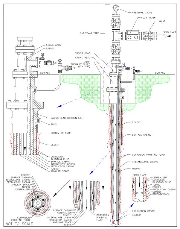
FIGURE 5 Typical Injection or Salt Water Disposal Well
